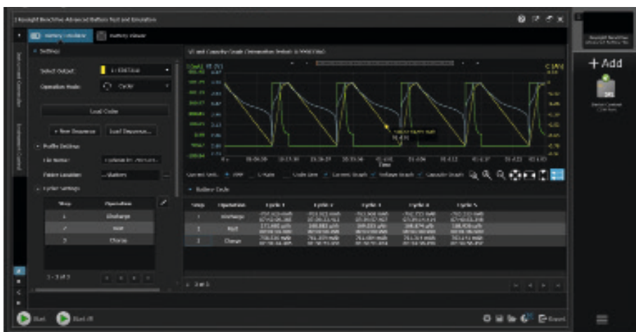
Figur 8. Battericyklning med mjukvaran BV9210B/11B PathWave BenchVue advanced battery test and emulation.
